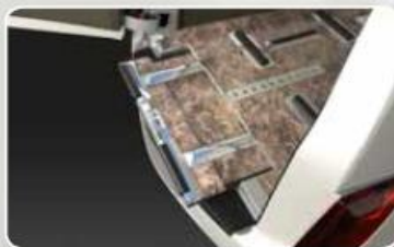
The Eagle Kingsley features a table extension which allows the casket to be loaded and unloaded without damage to the coach or casket.
